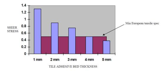
Another common error found locally is when the excess tile adhesive has not been removed from between tiles prior to grouting as per the SABS standard. Tile adhesive is relatively hard and it tends to transfer sheer stress from one tile to another. This results in huge sheer in the middle of the tiled room and tenting.
